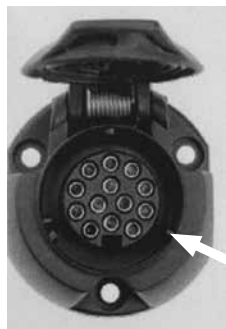
Fig. 5 - Socket body (containing female socket terminals) fitted to the car
