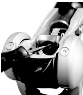
Fig 4. Remove head cap screw
