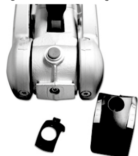
Fig 3. cheese head screw revealed
